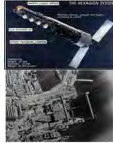
Figure 123: A list of US spy satellite programmes along with an image depicting KH-9 Hexagon, the last system, which relied on chemical film, and a computer-enhanced CCD-based KH-11 photograph showing the general layout of the Nikolaiev 444 shipyard in the Black Sea, with a Kiev-class aircraft carrier under construction<sup>237</sup>
